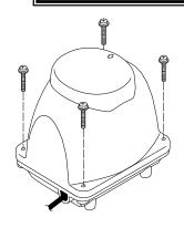
1. Remove cover bolts using a 8mm-box wrench.
