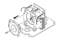
5. Remove nut and take a diaphragm off from a body.
