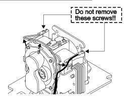
3. Remove a power cable from 3 hooks.
