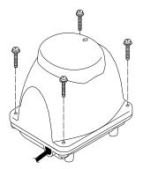
10. Fix cover bolts using a 8mm-box wrench.
