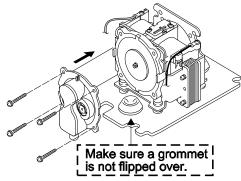
7. Insert a casing air outlet into a rubber grommet and fix a casing assembly with 4 screws.
