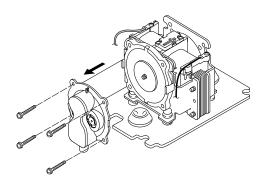
Remove 4 screws from a casing using a cross slot screwdriver.
